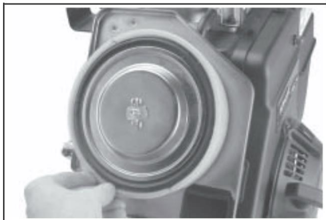
Figure 11-59. Installing Air Cleaner.
