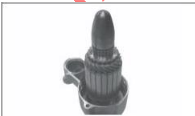
Figure 8-24. Tool on end of Armature.
