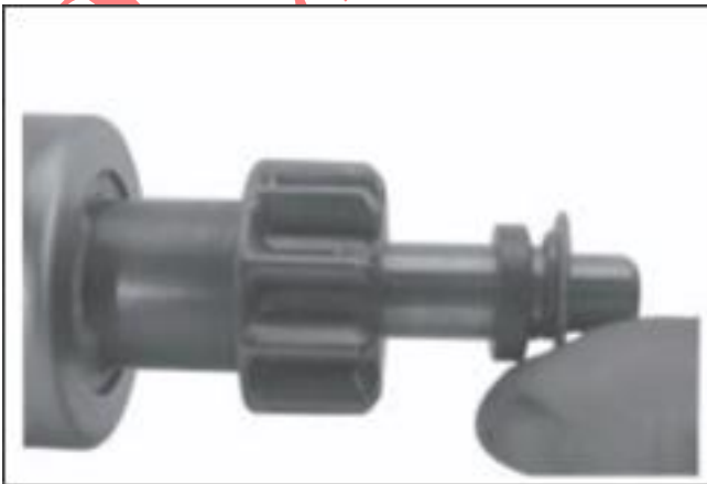
Figure 8-46. Thrust Washer Installation.
