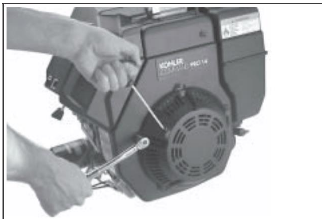
Figure 11-61. Installing Retractable Starter.
