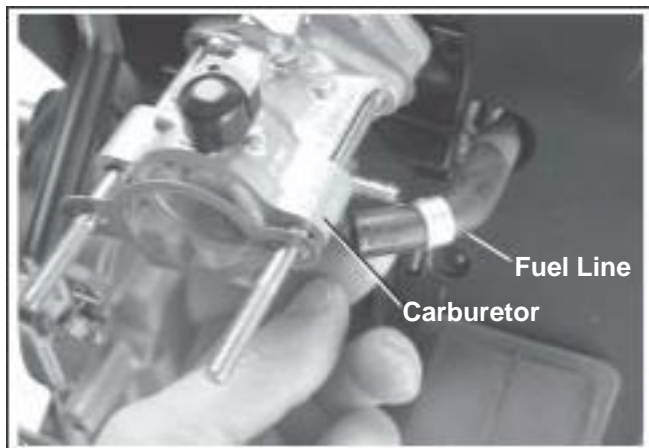
Figure 9-10. Removing Fuel Line From Carburetor.
