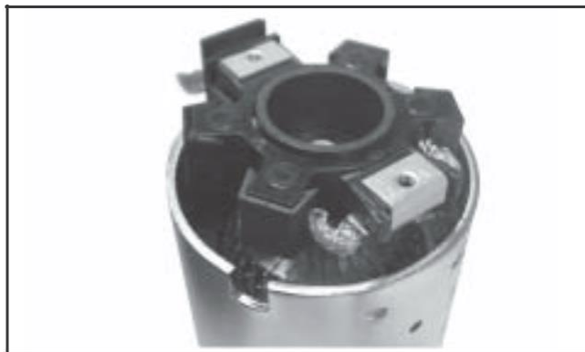
Figure 8-51. Installing Brush Holder Assembly with Supplied Tube.
