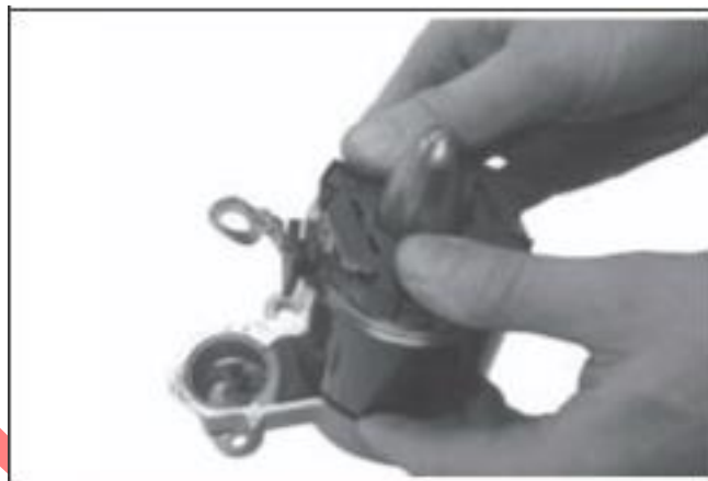
Figure 8-25. Installing Frame with Brush Plate Assembly.
