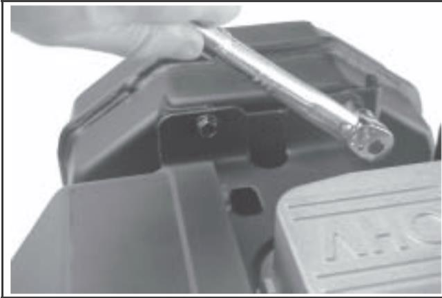
Figure 11-63. Installing Upper Muffler Bracket and Mounting Screws.
