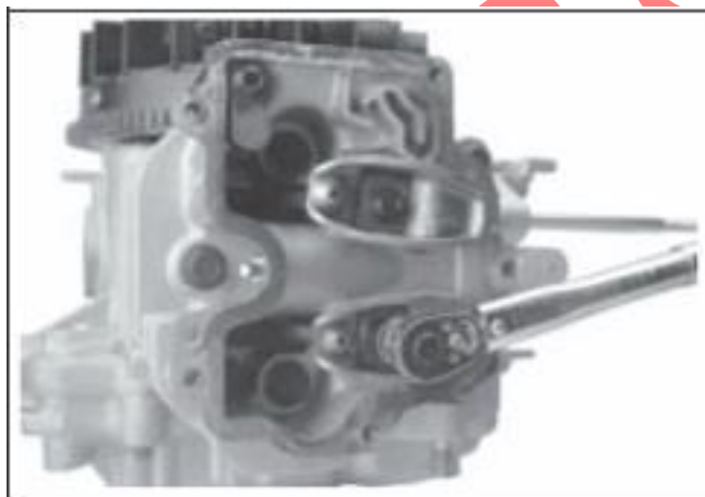
Figure 11-37. Torquing Rocker Screws.
