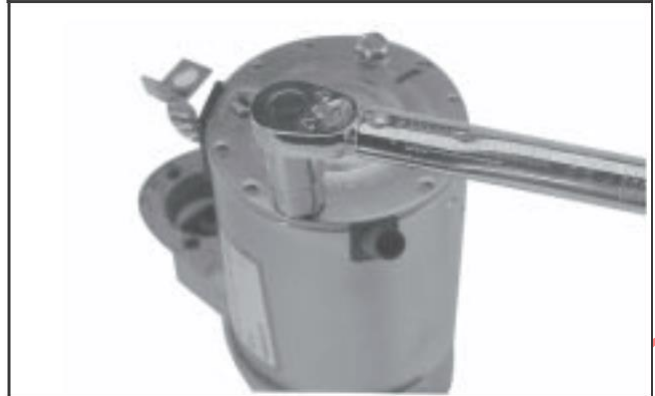
Figure 8-55. Torquing Thru Bolts.
