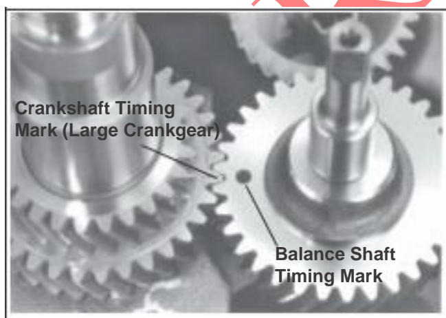
Figure 11-10. Aligning Timing Marks on Crank Gear and Balance Shaft Gear.
