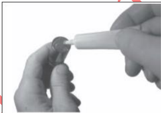
Figure 11-11a. Applying Camshaft Lubricant to Bottom of Lifters.
