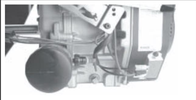
Figure 6-4. Oil Drain Plug Locations, Oil Filter, and Optional Oil Sentry™ Switch.
