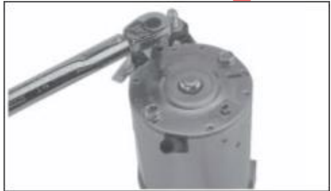
Figure 8-56. Torquing Brush Holder Screws.
