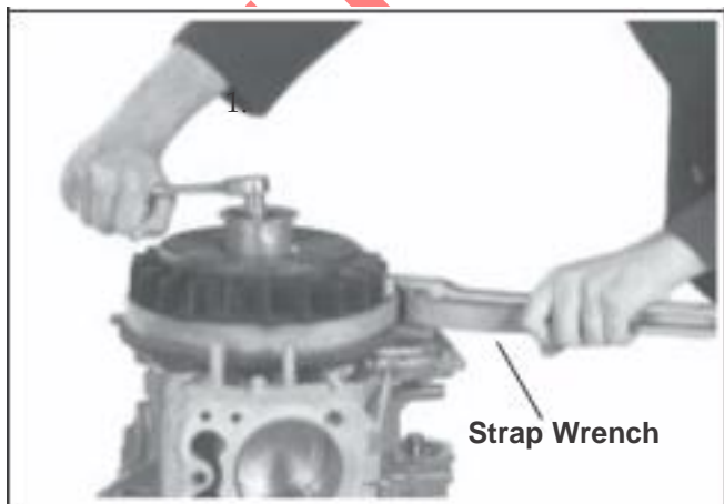
Figure 9-37. Removing Flywheel Retaining Screw and Drive Cup.
