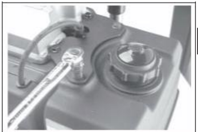
Figure 11-50. Installing Fuel Tank Upper Mounting Screws.
