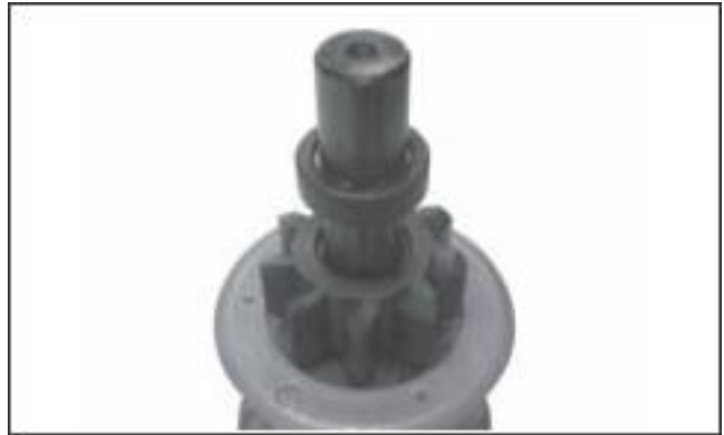
Figure 8-20. Lock Collar around Retaining Ring.
