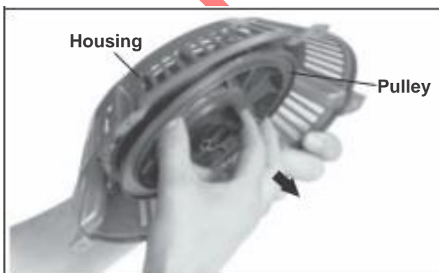
Figure 7-7. Removing Pulley from Housing.
