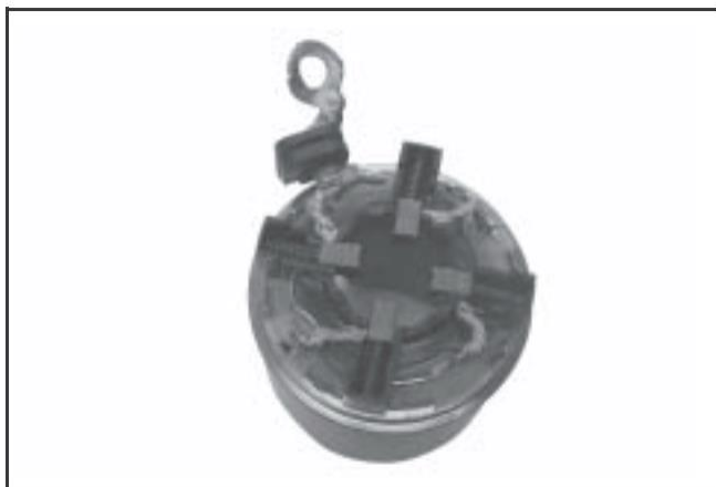
Figure 8-22. Mounting Brush Holder to Frame.
