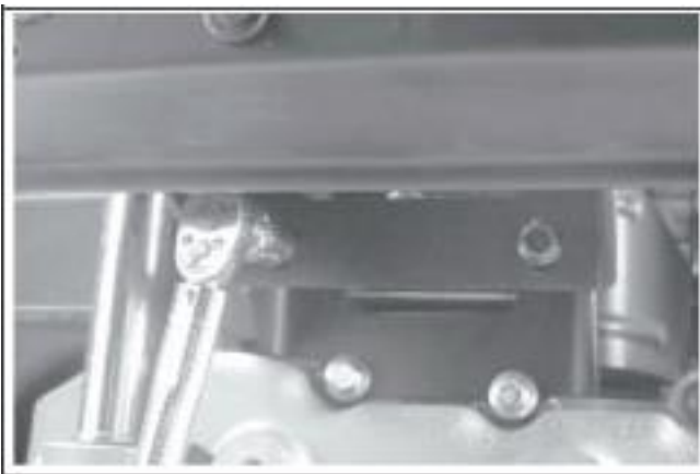
Figure 11-64. Installing Lower Muffler Bracket and Mounting Screws.
