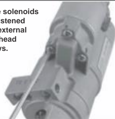
Figure 8-30. Removing Solenoid Screws.
