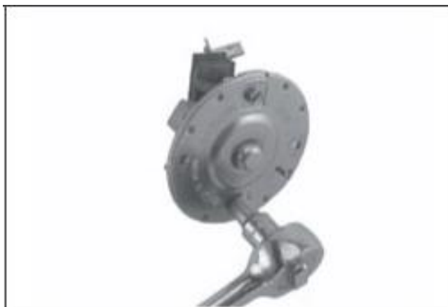
Figure 8-43. Removing Brush Holder.
