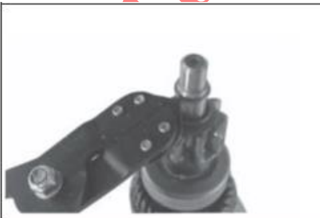
Figure 8-39. Removing Retaining Ring.
