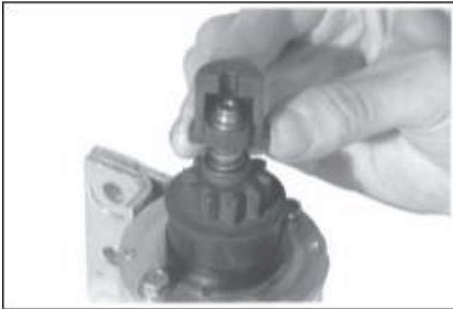
Figure 8-14. Assembling Larger Inner Half Around Spring Retainer.
