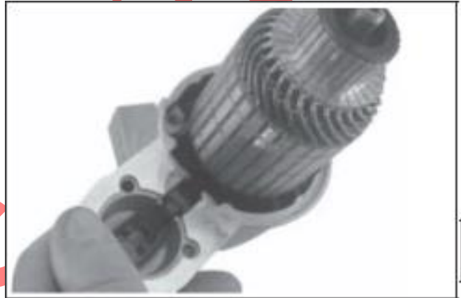
Figure 8-47. Installing Armature and Pivot Lever.
