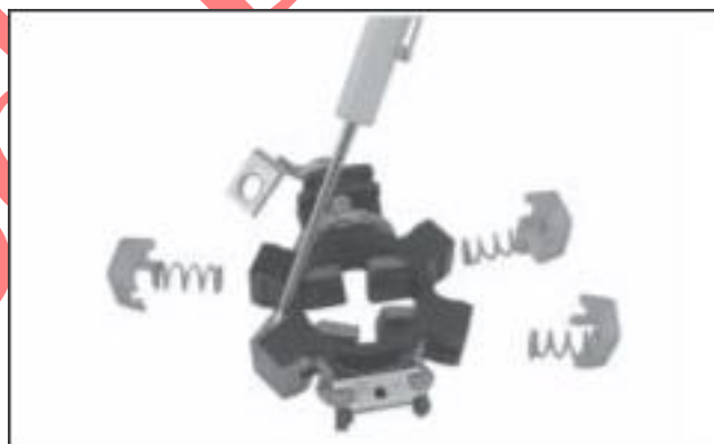
Figure 8-52. Removing Retaining Caps.
