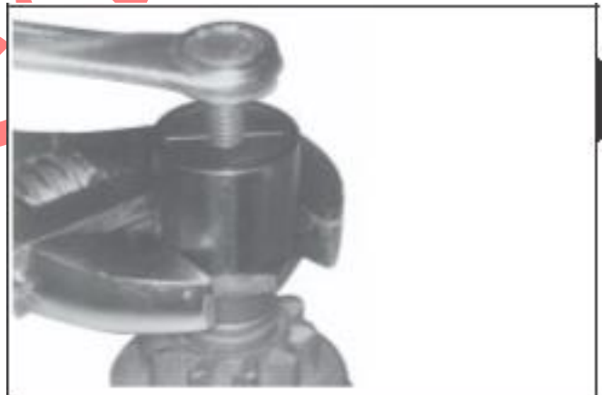
Figure 8-13. Holding Tool and Turning Center Screw (Clockwise) to Remove Retaining Ring.
