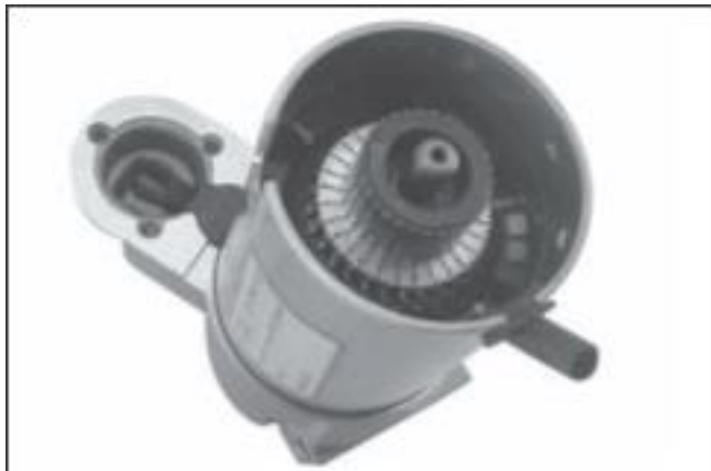
Figure 8-49. Installing Frame and Drain Tube.
