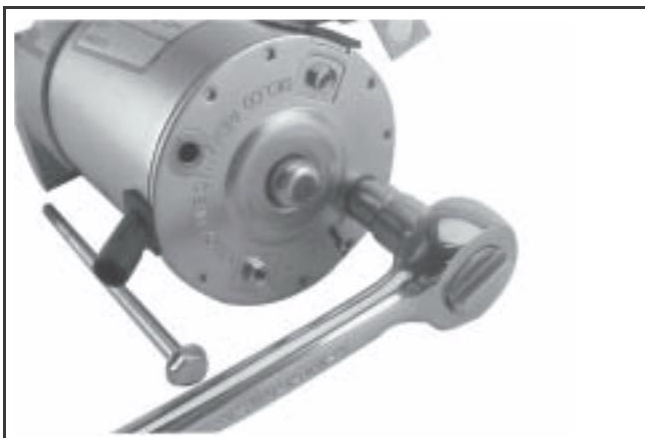
Figure 8-33. Removing Thru Bolts.
