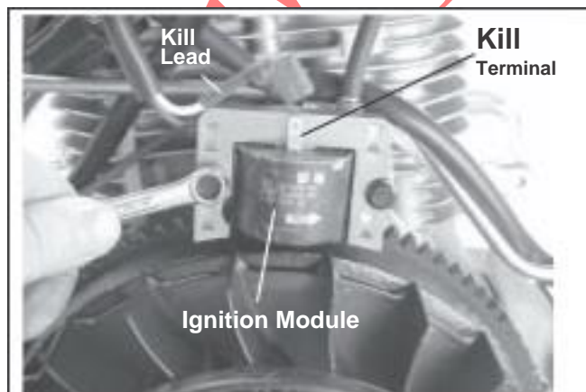
Figure 9-28. Removing Ignition Module.
