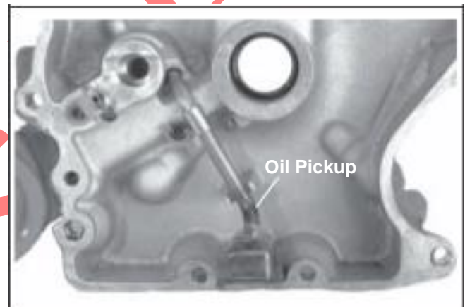
Figure 9-43. Removing Oil Seal and Pickup.
