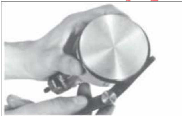
Figure 10-7. Measuring Piston Ring Side Clearance.
