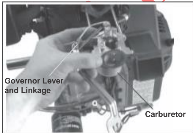
Figure 9-11. Removing Carburetor and Governor Lever.
