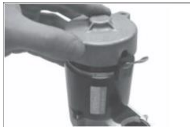
Figure 8-26. Installing End Cap.
