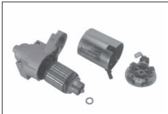
Figure 8-35. Starter Frame Removed.
