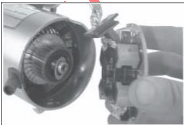
Figure 8-34. Removing Commutator End Plate Assembly.
