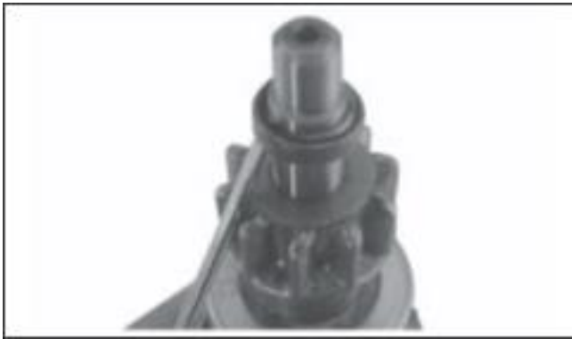
Figure 8-45. Installing Stop Collar/Retainer.
