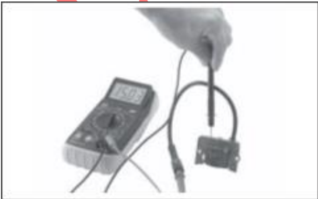
Figure 8-4. Testing Module Secondary.
