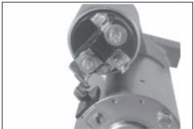
Figure 8-57. Positive (+) Brush Lead Connection.
