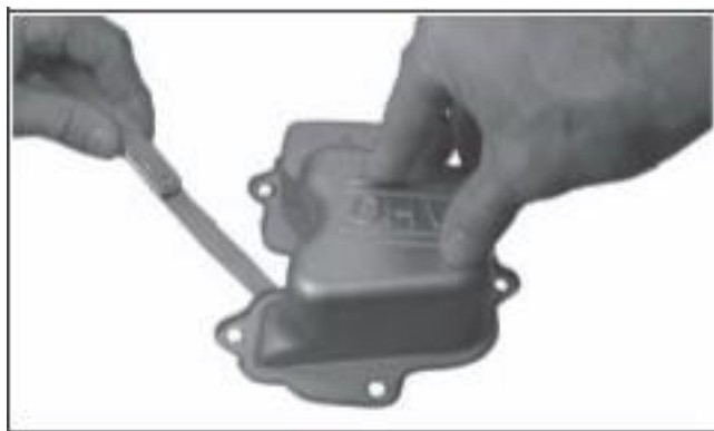
Figure 10-11. Checking with Feeler Gauge.
