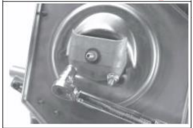
Figure 11-57. Installing Air Cleaner Base.
